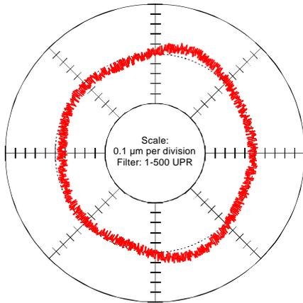
**Figure 3:** Trace of glass hemisphere used to check the scale error. The 1-500 UPR filter setting used here generally gives the highest noise level, represented by the “width” of the trace.
