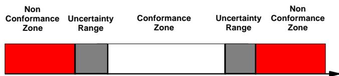
**Figure 2:** The Conformance Zone (white) is the tolerance reduced by the measurement uncertainty at each end. The Non Conformance Zones (red) are the areas outside the tolerance by more than the measurement uncertainty. The Uncertainty Ranges (gray) are the areas where conformance or non-conformance cannot be determined.
