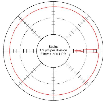
**Figure 4:** Trace of a Flick standard. Using the 1-500 UPR setting gives the least distorted trace of the standard.
