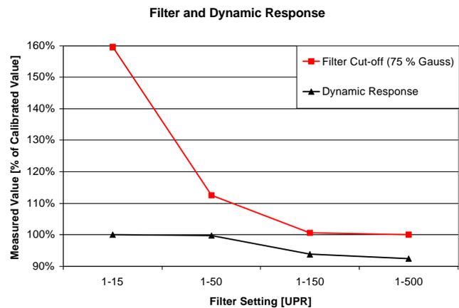
**Figure 5:** Typical deviation patterns for a non-standard filter and a limited dynamic response.
