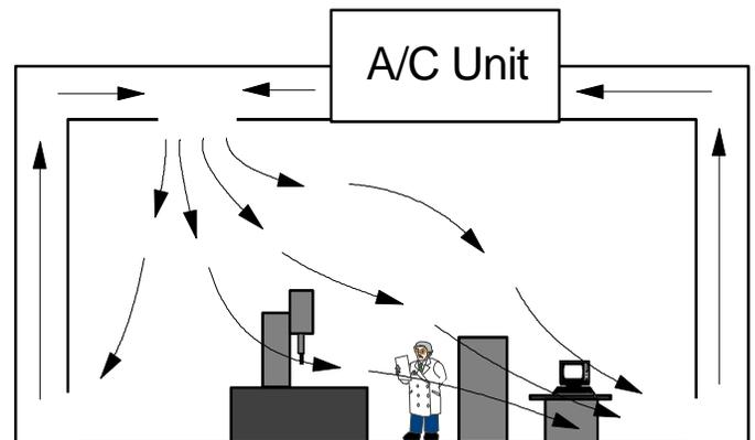
**Figure 2:** Example of a good laboratory layout. The air coming from the inlet in the ceiling passes over the CMM before reaching the operator, the control cabinet and the computer.
