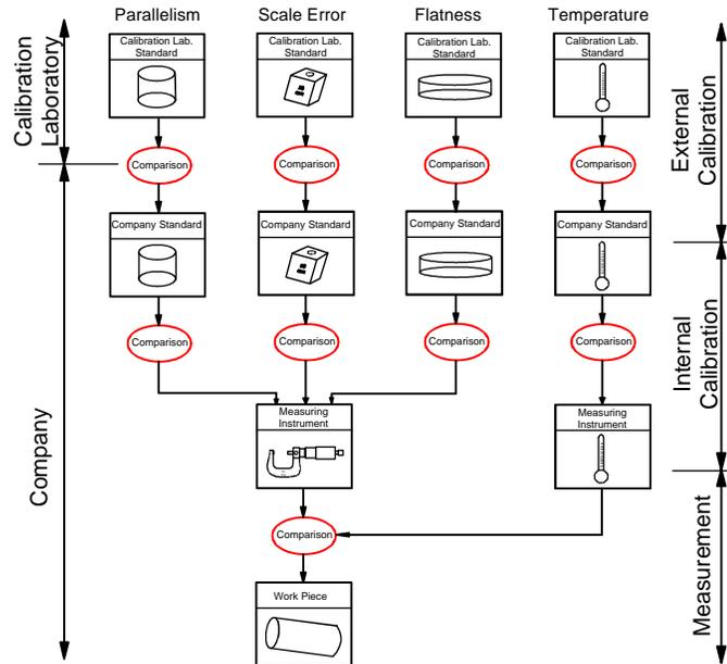
**Figure 1:** Traceability chains for a length measurement. The parallelism, scale error and flatness chains control the attributes of the micrometer, the temperature chain controls the conditions during the measurement. Each comparison represents a measurement or a calibration, linking an item to the item above in the traceability chain.
